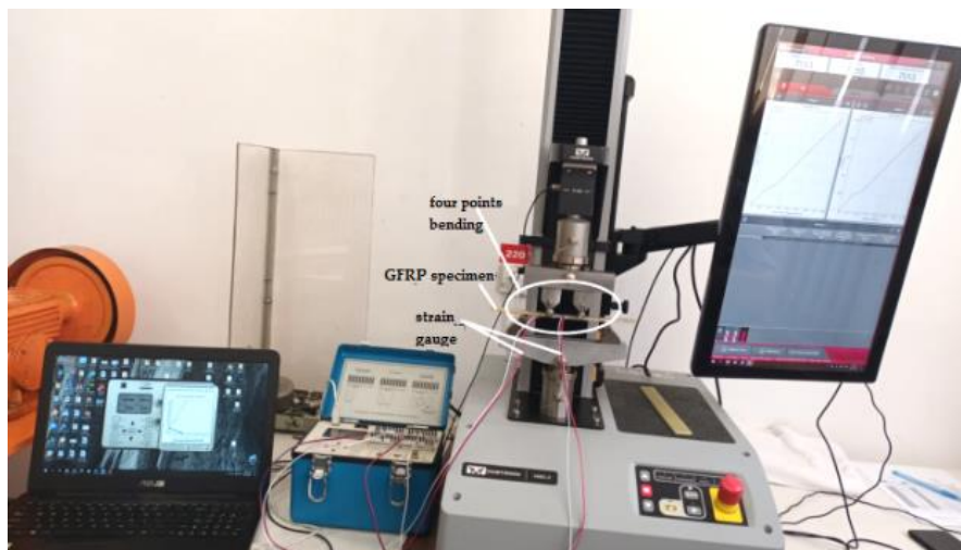
Fig. 7 – The experimental device for 4-point bending on the INSTRON 34SC-5 testing machine.
