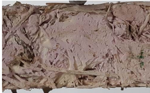
Fig. 1 – Hempcrete bricks produced by blending hemp shives with lime.
