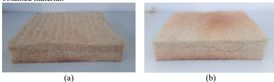
Fig. 1 – Heat-insulating non-woven fabric made of hemp and bi-component fibre.
