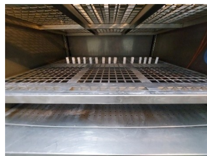
Fig. 7 – Positioning of the corian specimens in the climatic chamber used to determine the compressive strength under freeze-thaw cycles.
