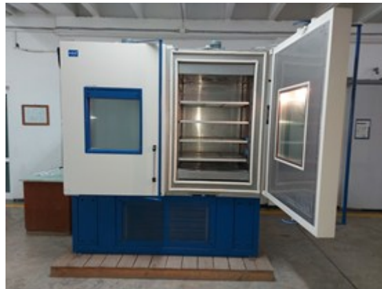
Fig. 1 – Feutron Klimasimulation GmbH - Twin test climate chamber - Test device.
