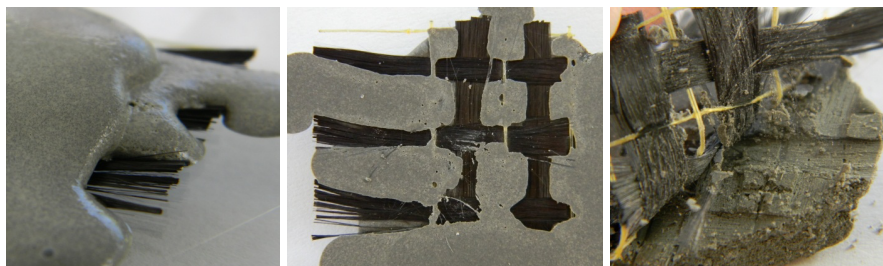
Fig. 5 – Modified mineral matrix with bidirectional reinforcement.
