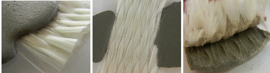
Fig. 3 – Modified mineral matrix with unidirectional reinforcement.
