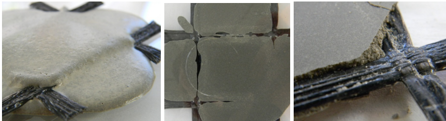
Fig. 8 – Modified mineral matrix with bidirectional mesh.
