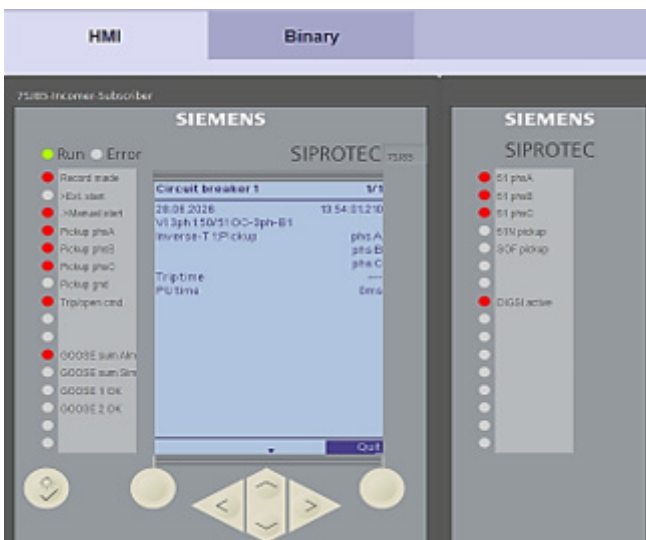
Figure 5: Relay HMI response, displaying the inverse-time overcurrent protection pickup across three phases.
