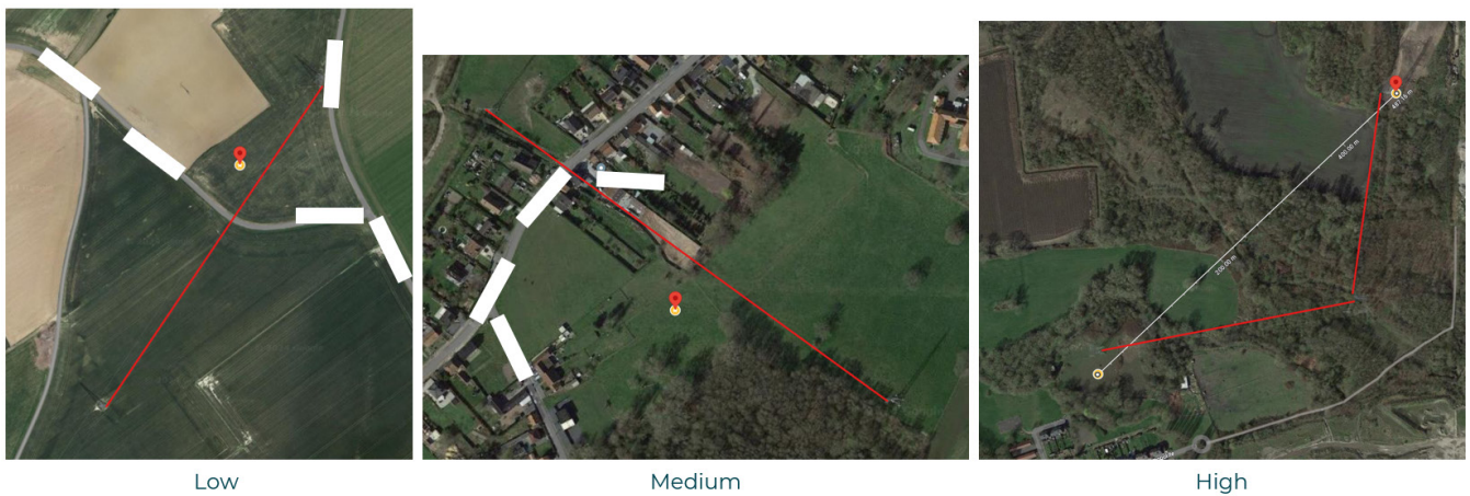
Figure 4: Wind obstruction categories (view from maps.google.com). Line route is highlighted in red
