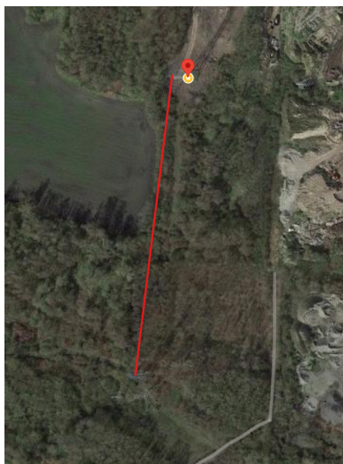
Figure 15: One span, highlighted in red, in a forest corridor that shelters the wind (view from maps.google.com)
