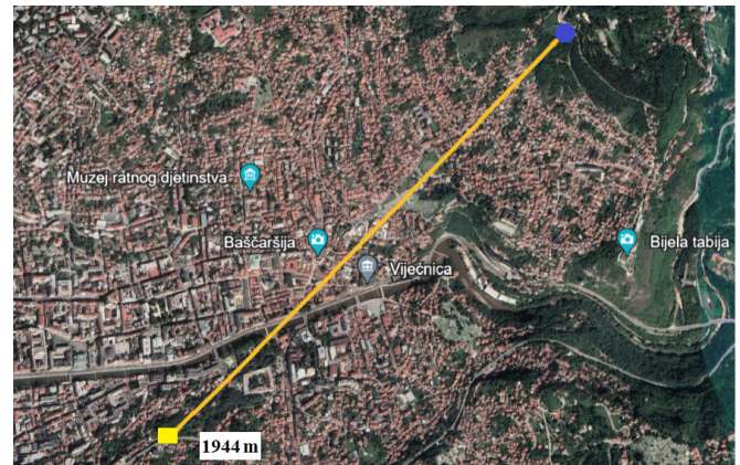
Figure 7: Link range measurement in an urban area in the case of a clear line of sight
