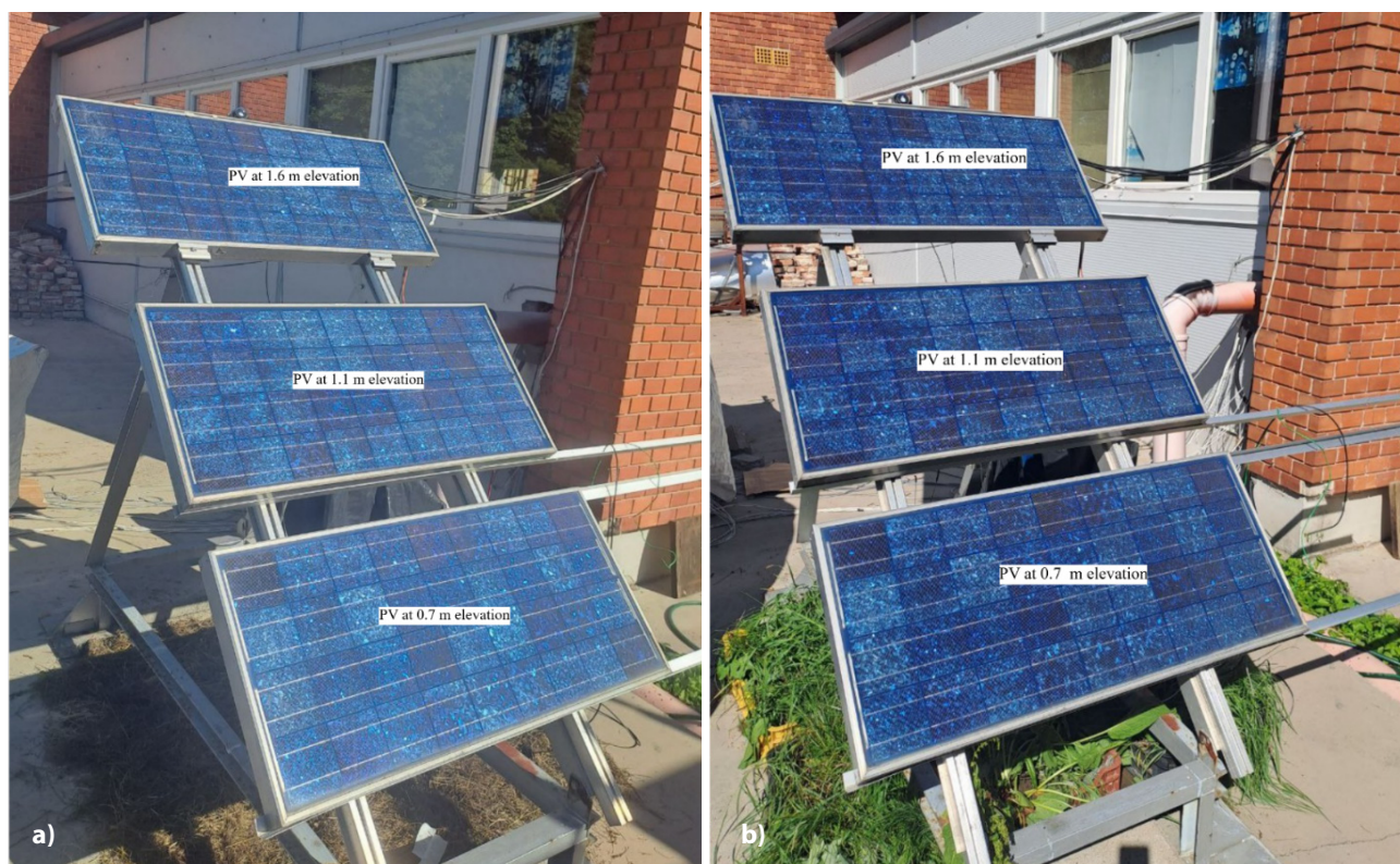
Fig. 3 Covering the PV module ground with: a) dried grass; b) vegetation
