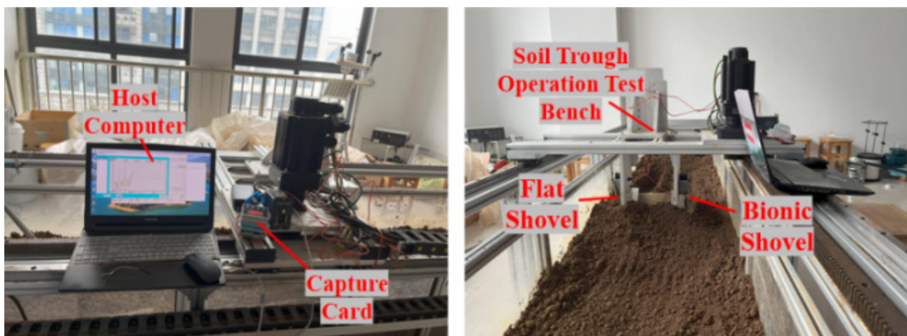
Fig. 18 Soil trench test environment
