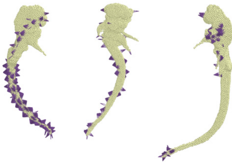
Fig. 16 Comparison of bond states after root and rhizome are excavated by the excavating shovel (a) Initial state; (b) After planar excavation; (c) After biomimetic excavation
