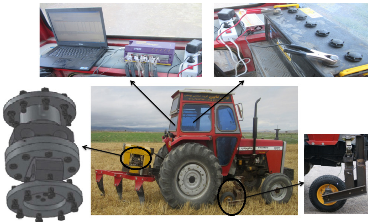
Fig. 4 Three-point-hitch dynamometer and data acquisition system inside the tractor cabin
