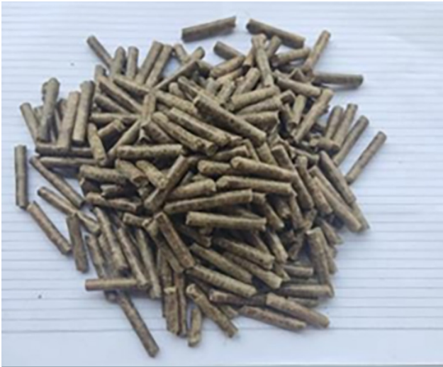
Fig. 6 Sorghum biopellet products by vertical pelletiser
