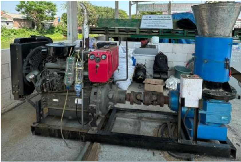
Fig. 2 Prototype of a roller-type biopellet raw material pelleting machine
