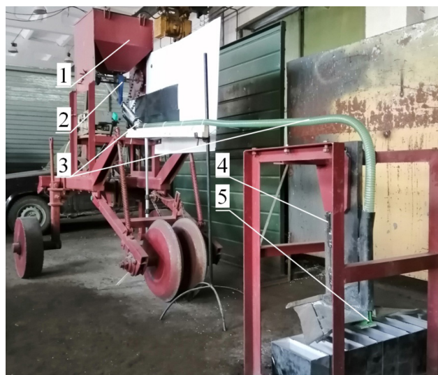
Fig. 5 Laboratory-field setup for subsurface application of granular mineral fertilisers with a variant of the flat-cutting working body
