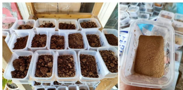
Fig. 4 Drying and grinding soil samples
