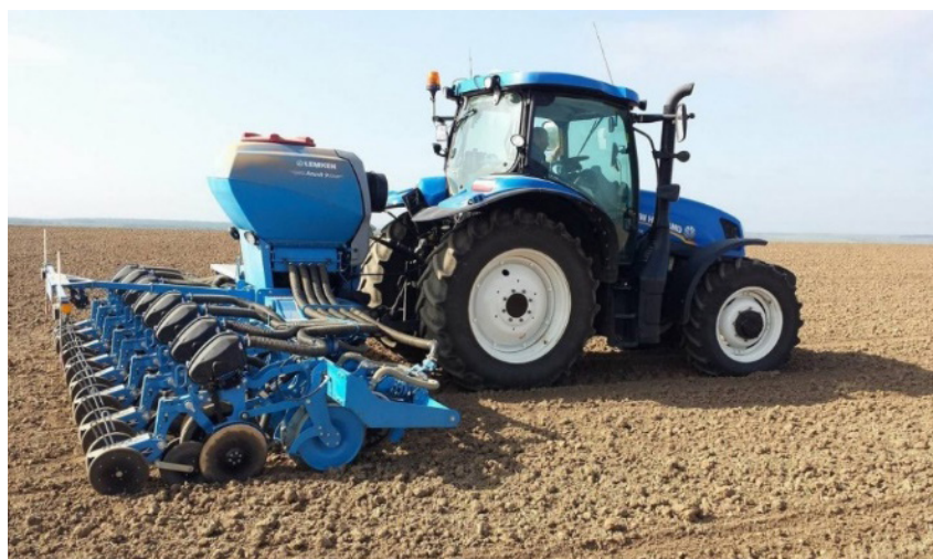
Fig. 2 Machine-tractor aggregate for staggered sowing of hoeing crops Source: Agronika, 2024
