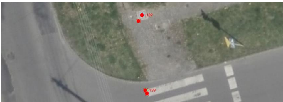
Figure 1. Example localisation of different type control points in selected options of experiment methodology
