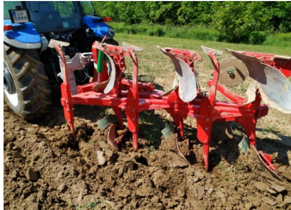
Figure 2. View of agricultural tractor with modernized plough during field test
