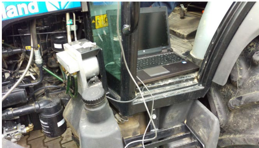
Figure 5. the fuel flow meter mounted on the tractor.
