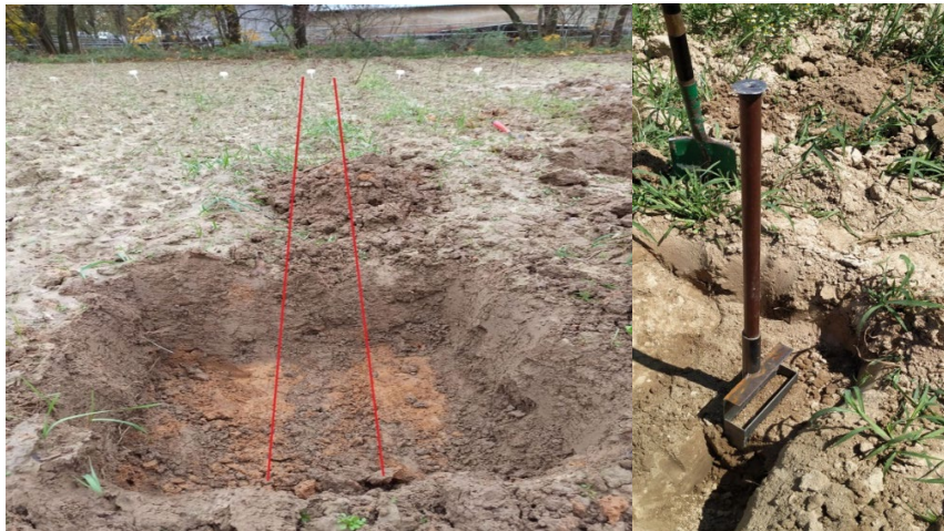
Figure 7. the soil outcrop and device for collecting rectangular soil samples
