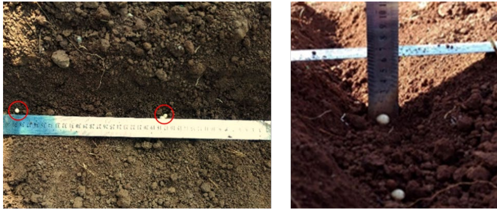
Figure 14. Method for measuring inter-row seed spacing and planting depth using a steel ruler
