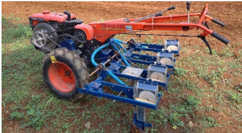
Figure 13. Prototype of the vacuum-type soybean seeder mounted on a walking tractor, prepared for field testing
