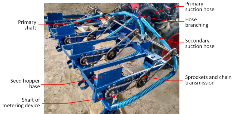
Figure 9. The arrangement and position of the primary suction hose and secondary suction hoses
