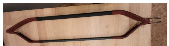
Fig. 1 Stator coil with semiconductive coating (Brown)
