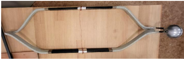
Fig. 2 Stator coil without semiconductive coating (White)
