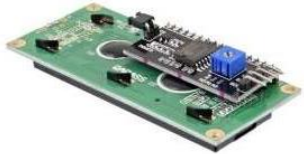
Fig. 4 PCF3874 module for LCD display
