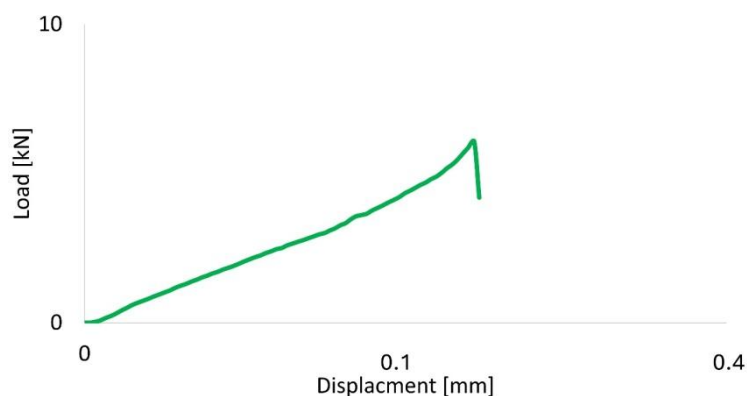
Fig. 6. Load-displacement curves were obtained during uniaxial compression testing of Al 2 O 3 -Cu-Cr composite systems containing a 2.5 vol.% metal phase
