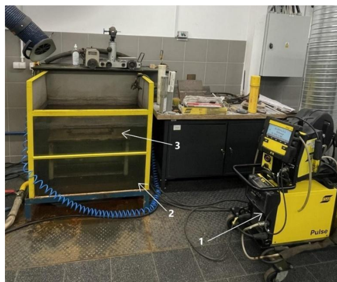
Fig. 1. View of the underwater welding stand used in the experiments: 1 – welding power source, 2 – tank with water, 3 – welding table
