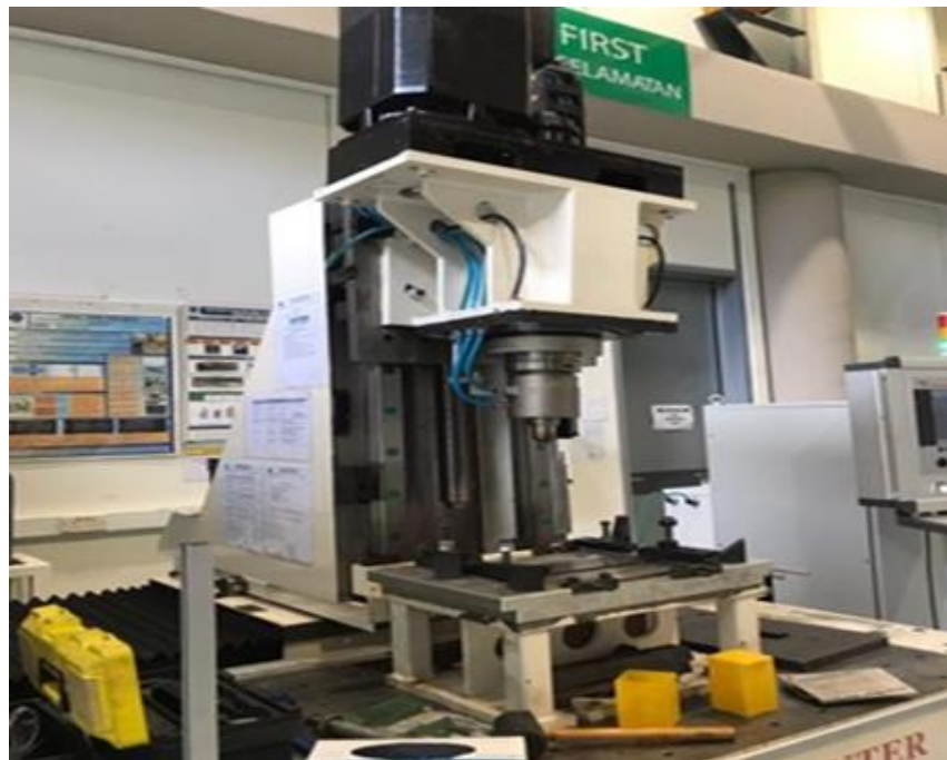
Fig. 2. Friction stir welding machine (FSW-TS-F16 model)
