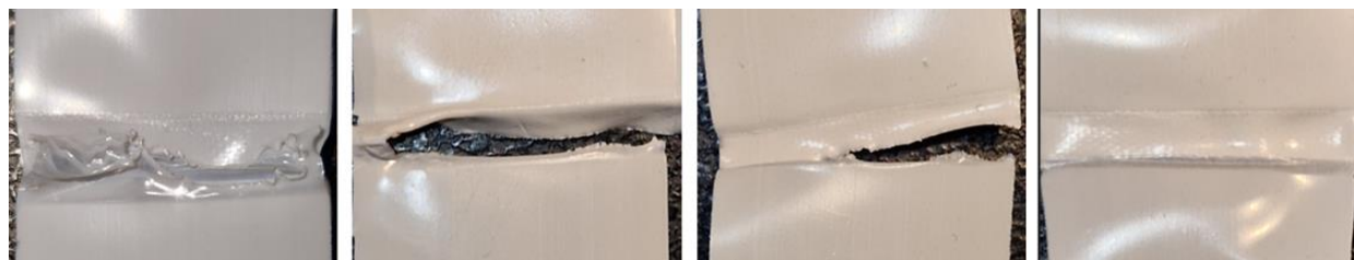
Fig. 5. Welds of film samples after Hot tacktesting, from the left: RE pure, RPE 60, RPE 80, RPE pure
