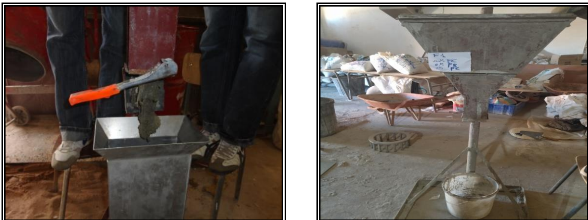
Fig. 9. Example of V-funnel flow time for fresh SCSC (formulation F1)
