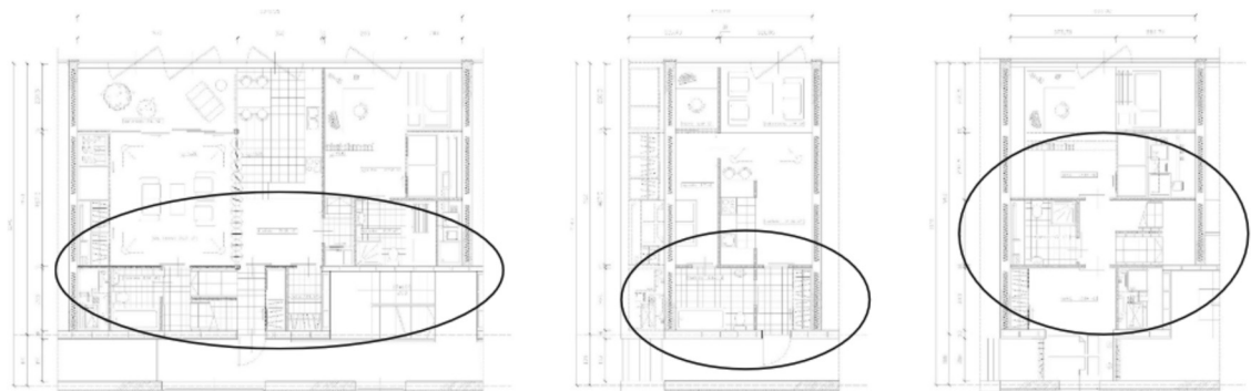
Figure 6. The apartments function as heat exchangers, working together with buffer zones to form a thermal accumulator model. Own elaboration based on an academic design project (project author: Adam Myczkowski; design studio supervisor: Associate Prof., Eng. Arch. Jerzy Wojewódka; course instructor: Associate Prof., Eng. Arch. Grzegorz Nawrot).
