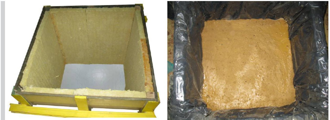
Figure 1. Test bench: a) damping of the side walls with mineral wool, b) view of the clay layer with foil protection
