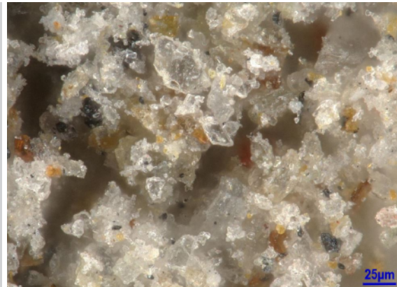
Figure 1. Digital microscope image of the tested basalt dust (1000x magnification)
