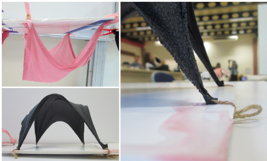
Figure 1. Physical form-finding workshop: funicular membranes using fabric and candle wax
