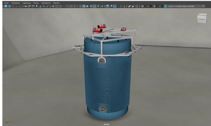
Fig. 5: 3D model of the container and conceptual prototype of a mobile radiation measurement system in Autodesk Maya
