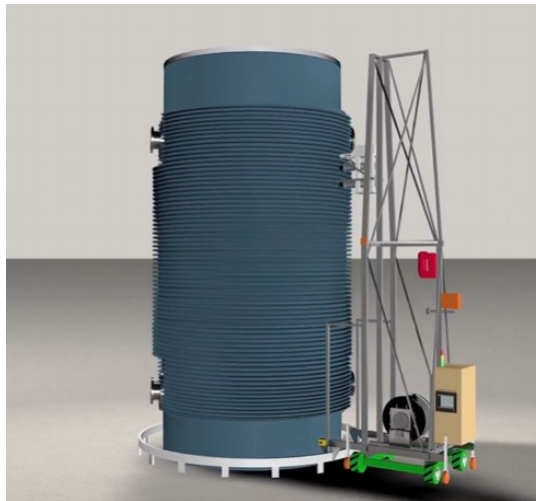
Fig. 1: Castor 440/84 and existing mobile radiation measurement system
