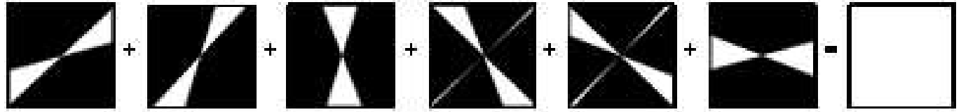
Figure.1 In PPFC, FDFB (with six directional filters) divides the frequency spectrum without leak
