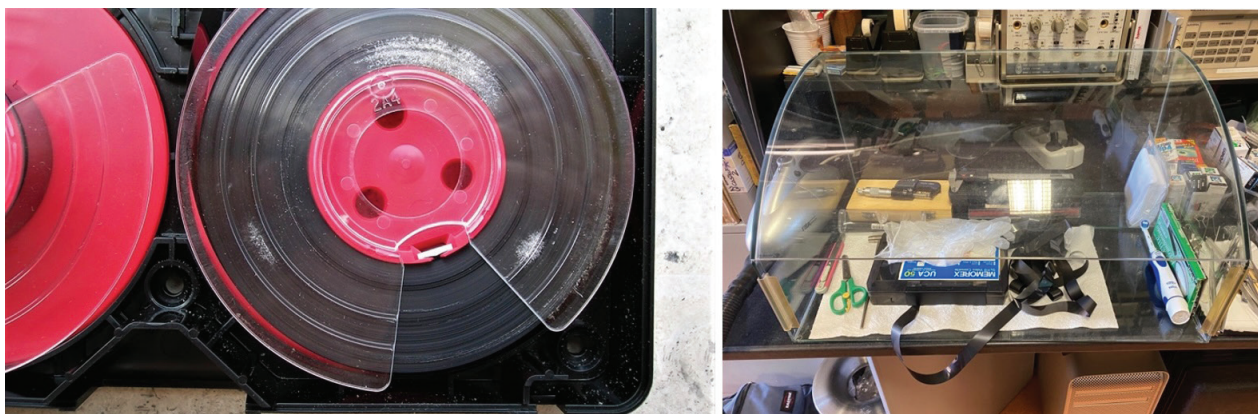
Figure 2. On the left, a U-Matic cassette tape contaminated by mould (photo by G. Coassin). On the right, Coassin's homemade cleaning box (photo by S. Minniti).
