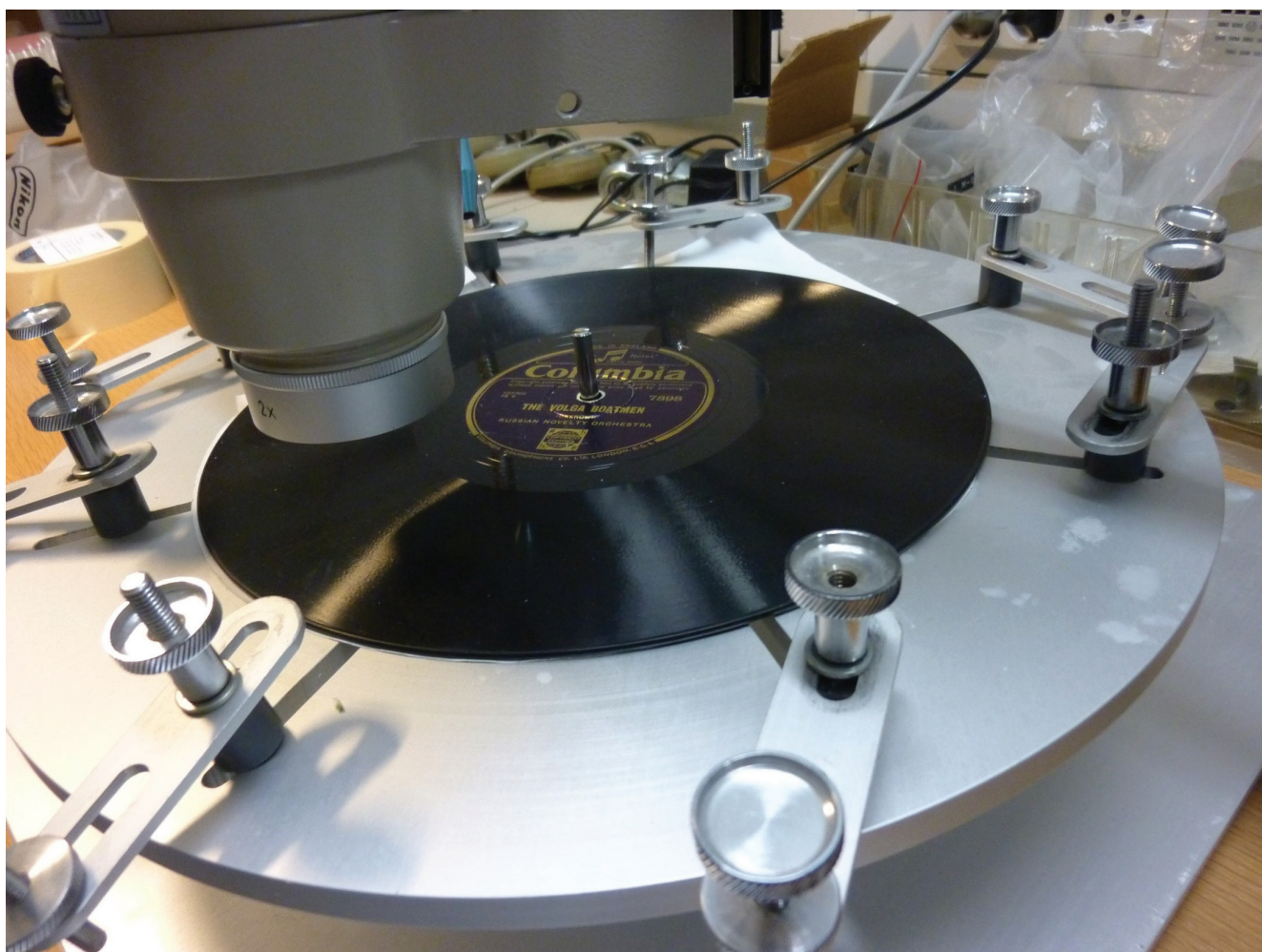
Figure 6. Audio restoration tools of the Yle audio archive's restoration studio included a microscope which enabled observation of the grooves of shellac records. Nowadays, a lot of signal manipulation can be done in the digital domain, for example a coughing member of the audience can be removed from a concert recording afterwards if necessary. Photo: author.
