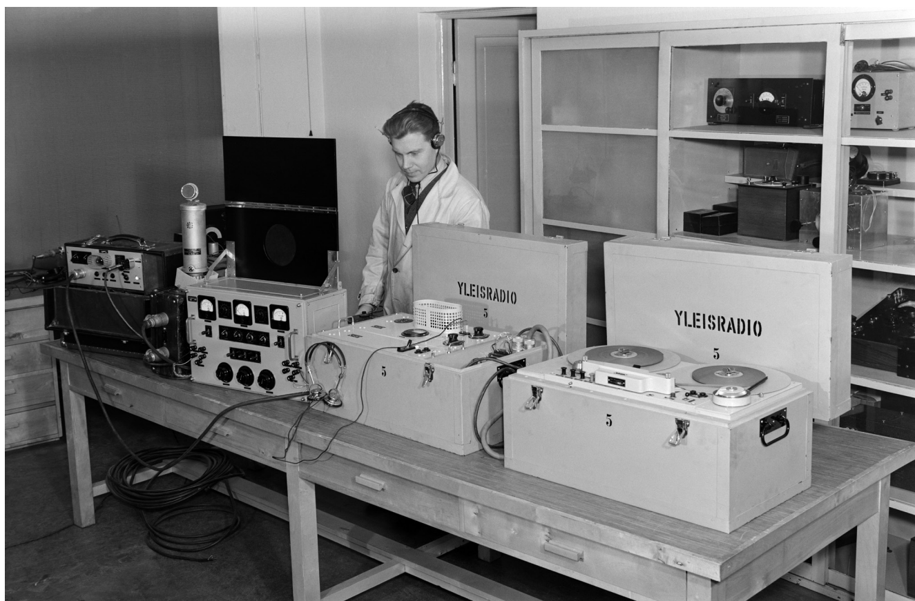
Figure 3. Yleisradio's in-house engineering manufactured power supplies, amplifiers and transformers which are combined with Telefunken microphone and AEG tape recorder to constitute a recording unit for the 1940 Olympic broadcast, Date: pre-1940. Photo: Yle Photo Archives.
