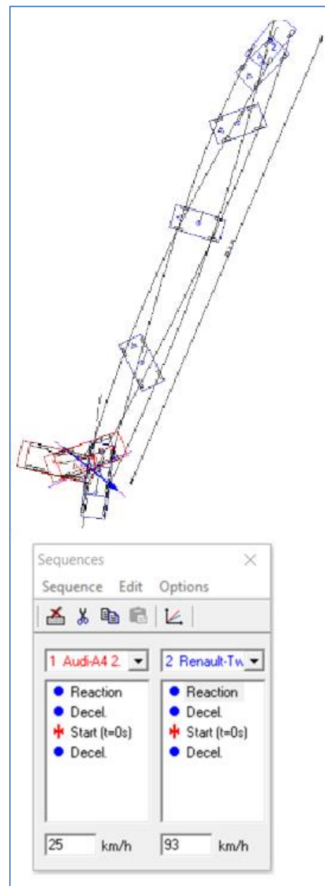
Fig. 3 PC Crash simulation and calculation of velocities of vehicles
