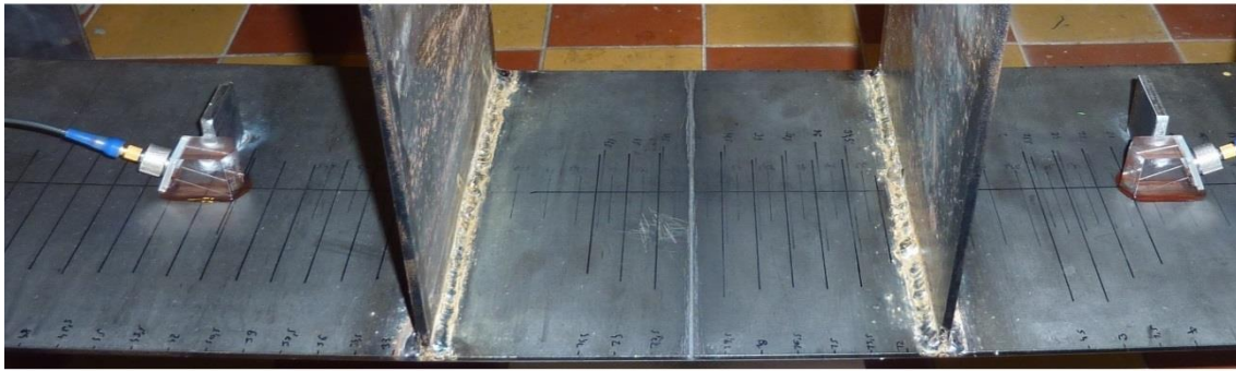
Fig. 11 Model position of transducers on the sample for the transmission measurement method
