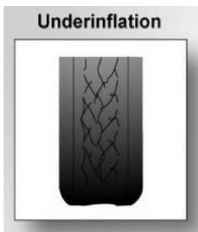
Figure 1. Wear due to under inflation ( https://www.rv.net )
