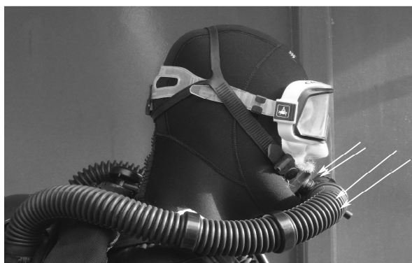
Fig. 2. Respiratory loop of a rebreather (the authors' own photos). The arrows show the directions of additional forces during movement in water.
