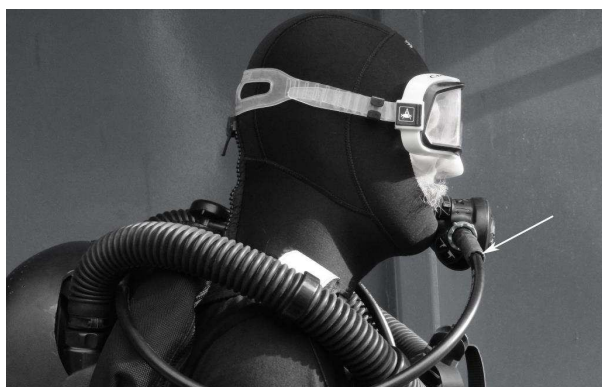
Fig. 1. Rebreather – open circuit (the authors' own photos). The arrows show the directions of additional forces during movement in water.
