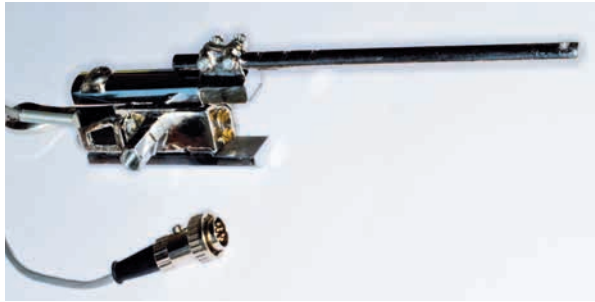
Fig. 1. ADInstruments computer-controlled pressure sensitive device
