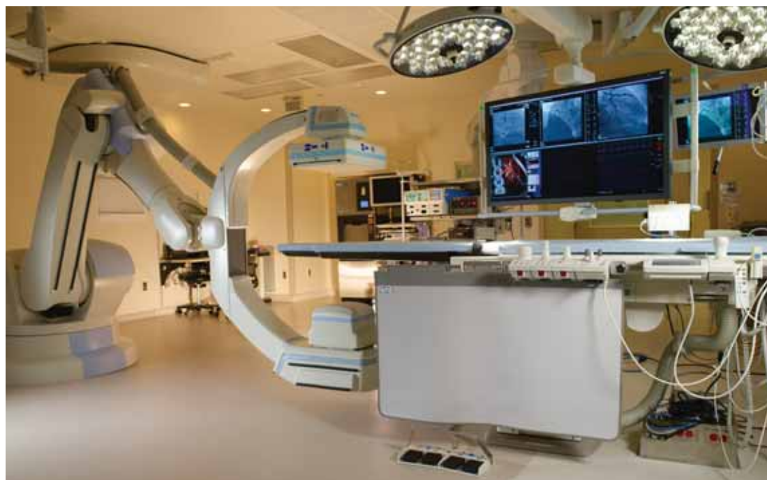
Figure 7. The modern hybrid suite at The Methodist Hospital. In addition to regular fluoro capabilities, the new Siemens fixed unit (DynaCT) located in the suite features rotational 3D angio/CT capabilities with fusion technology. The monitors can show the patient's vital data, real-time fluoro, IVUS images, previous CT and angio studies, and real-time road mapping.
