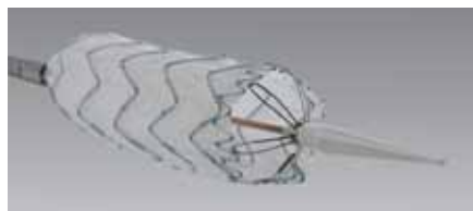
Figure 6. Talent™ thoracic stent graft with the Captivia® delivery system. The proximal bare metal stent is constrained in the delivery system to be released independent of device deployment. Image courtesy of Medtronic, Inc.
