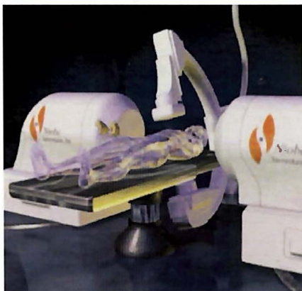
Figure 1. The permanent magnets are shown as they would be positioned around a patient in a cardiac cath lab. When not in use, the magnets are mechanically withdrawn away from the procedure field.
