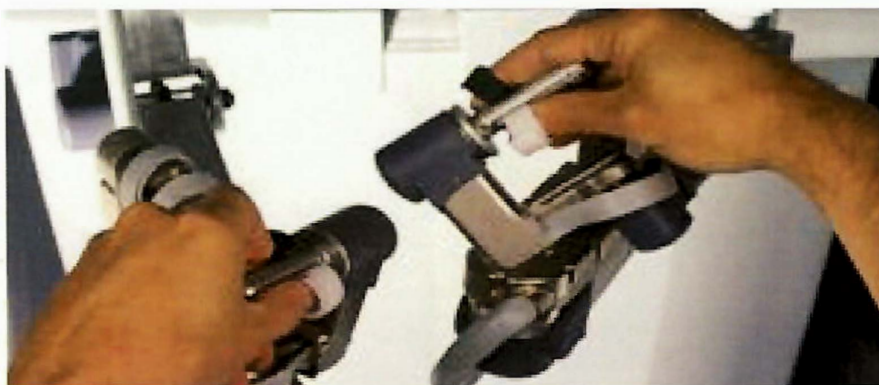
Figure 5. Using the two toggles mounted on the surgical console, the surgeon can transmit all his finger, hand and wrist movements to the instruments within the chest.
