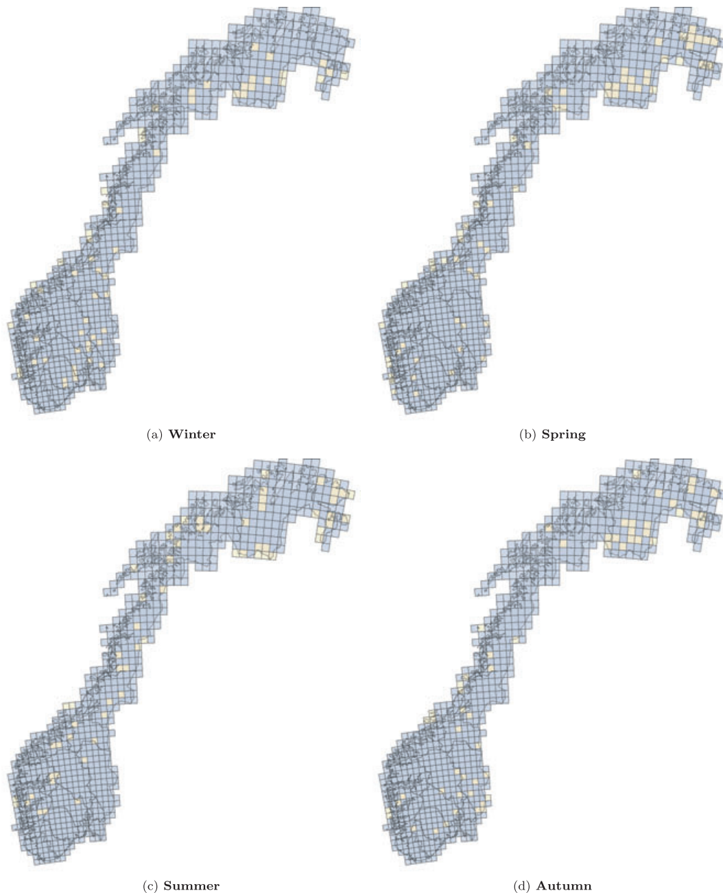
Fig. 3. Kolmogorov–Smirnov two-sample test used with a significance level \alpha = 0.05 . When there are no significant differences, a grid cell is yellow, that is, p\text{-value} > \alpha . If the p\text{-value} \leq \alpha the grid cell is blue.
