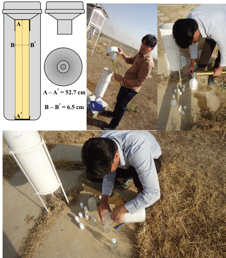
Fig. 3. The schematic picture of a rainwater collector and the procedure for sampling the stable isotopes.
