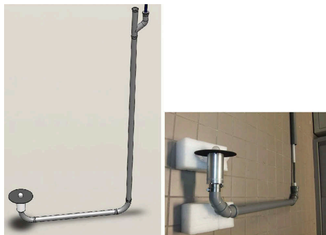
Fig. 2. Scheme of the apparatus developed for measurements of spectral underwater solar irradiance. Detail of the optical receiver and multilayer protecting frame of underwater device for measuring downwelling spectral irradiance.
