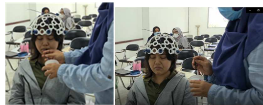
Fig 3. The EEG signal recording process during the insertion of sour taste stimuli
