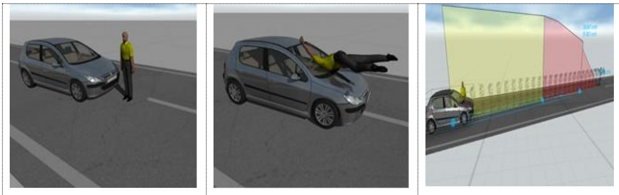
Fig. 6 Test-simulation of crash “Adult pedestrian- Peugeot 307”
