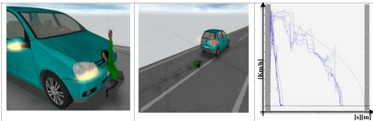
Fig. 7 Test simulation of crash “Adult pedestrian - VW Golf V”
