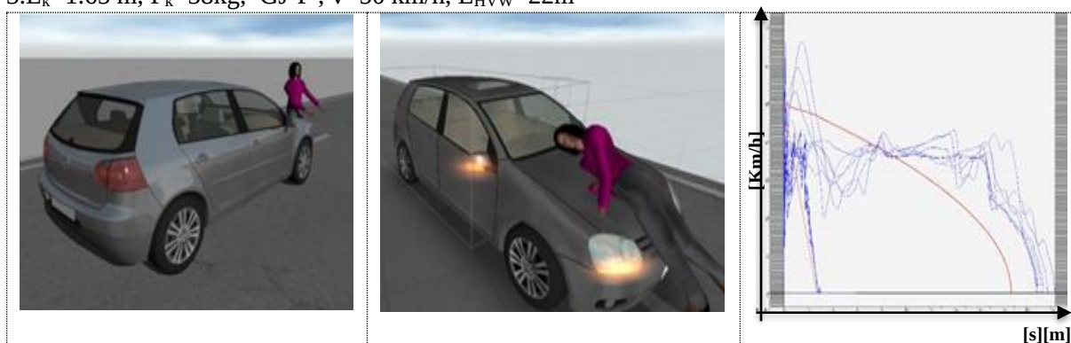
Fig. 9 Test simulation of crash “Adult pedestrian- VW Golf V”
