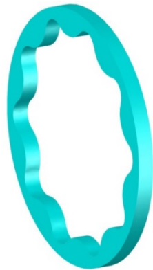
Fig. 16 – A conceptual view on 3D CAD model of a cycloidal gear having the transverse section the 2D profile from Fig. 12.
