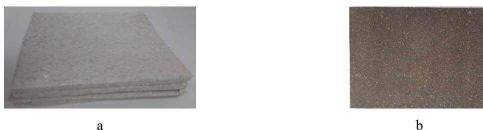
Figure 2. Thermobonded nonwoven stack (a) and composite material made therewith (b)
