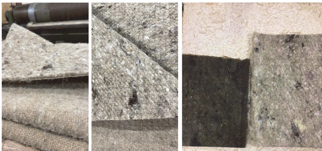
Figure 5. Irish Wool and Hemp comingled on the right hand side with the bio resin added on the sample to the left (darker brown) Image: Chris Weiniger
