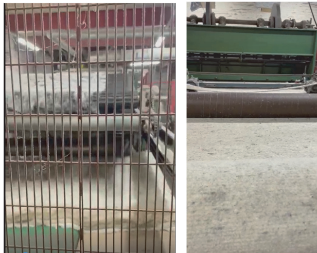
Figure 4. Preparation of 60/40 Irish Wool Hemp for Non-woven fabric for testing with the bio-resins. Image: Chris Weiniger
