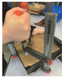
Figure 12. Placing the sample on the mold block
