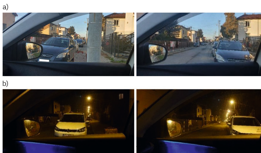
Fig. 1. Road visibility by a driver joining the traffic from a minor road a) during the day, b) at night (photo by author)
