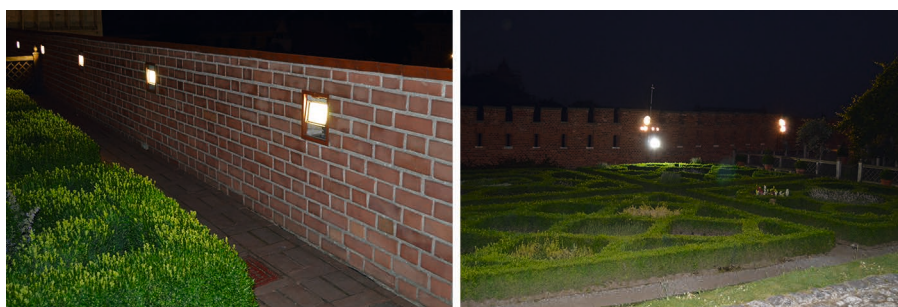
Fig. 30. Example of glare caused by headlights located in the lower terrace of Royal Gardens (by Jakub Łygan)
